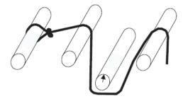
Tighten the rope with the calibration weight when weight calibration:
